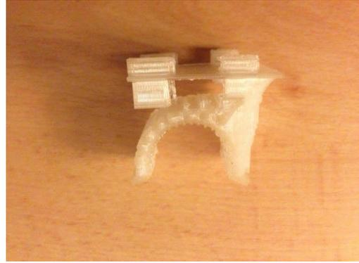
Fig. 8 (right): Plastic flute attachment for MiniBee sensor (Moroz, S.)
